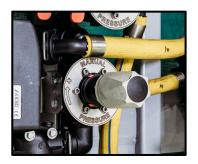
Flow not utilised for Agitation will continue through the Manual Flow Regulator Valve. This sets the maximum available pressure the valve set can deliver.
