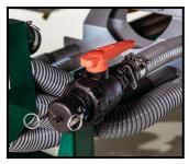
Filling is done via a 2 inch camlock that allows the operator to connect the Air Seeder to an external source and simply pump the fluid in via an external pump. It is recommended that additional filtration be considered so as to avoid any contaminates from entering the main supply tank.
