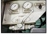
The Pump Pressure Tap can also be used to reset the flow limiting valve
