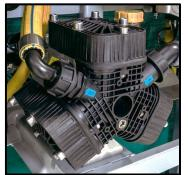
The Bertolini Pump is a diaphragm pump. The diaphragms and valves can be damaged without proper filtration and care. It is recommended that the filtration elements are serviced regularly and that the system is regularly flushed with clean water.
