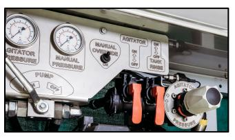
Different agitators are available for differing uses. Simplicity fits the 2.5mm orifice as standard. With this orifice fitted the agitator will roll 600 litres of tank mix every minute if pressure set at 5 bar, or 72.5psi. At this setting the agitator is only drawing approximately 7 litres per minute from the pump.
