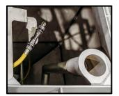
An overflow tube is fitted on the inside of the tank. Should the tank be overfilled the excess fluid overflows through this tube onto the ground.
