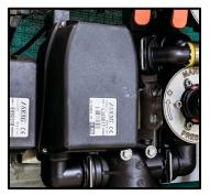
Once through the pressure filter, flow enters the dump valve. The dump valve works inversely to the Section or delivery valve, so when the section valve is closed, dump valve is open back to the return circuit, allowing all pressure flow back to the return circuit.
